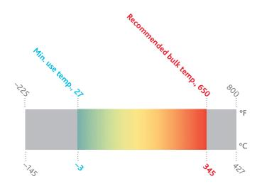
Eastman Therminol® 66 heat transfer fluid offers outstanding high-temperature performance to 345°C (650°F), including excellent thermal stability and low vapor pressure. These properties result in reliable, consistent performance of heat transfer systems over long periods of time. Therminol 66 performance is proven through many years of industrial experience under a wide range of operating conditions. No heat transfer fluid material in the world has had more success than Therminol 66.
